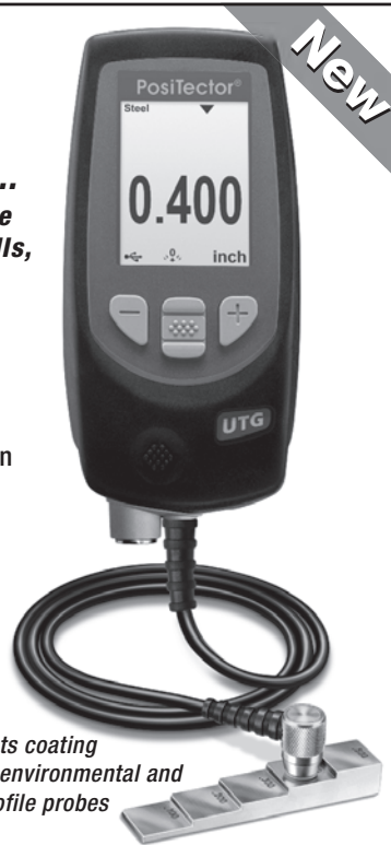
UTG M Thru-Paint models measure the metal thickness of a painted structure without having to remove the coating.
