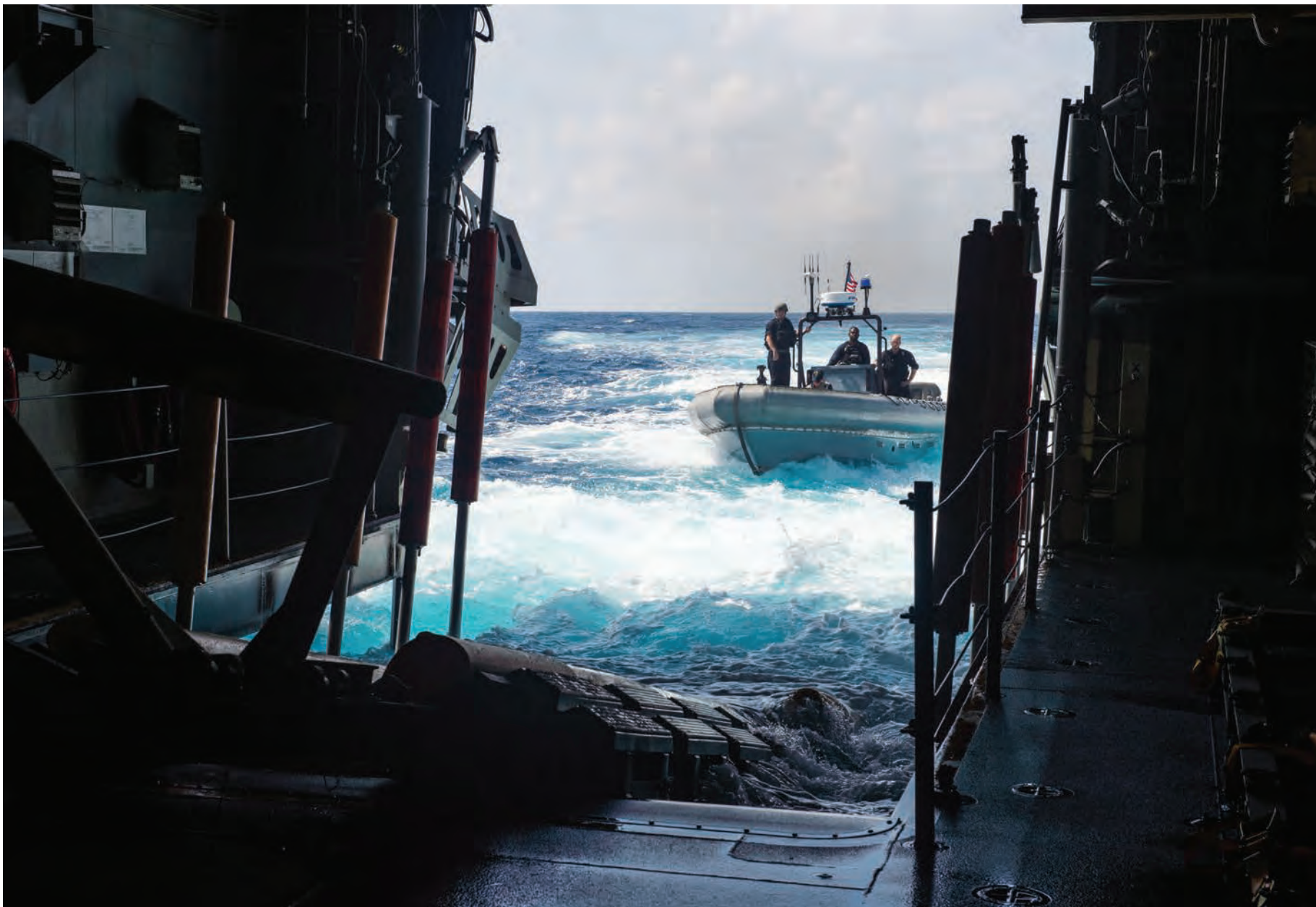
An 11 meter rigid hull inflatable boat (RHIB) approaches the open stern doors of the water borne mission zone aboard the USS Fort Worth (LCS 3).
