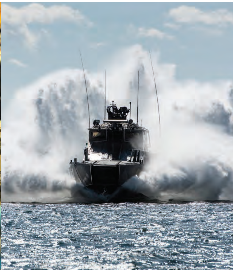
The stop distance from full speed, up to 50 knots, is only 60 m.
