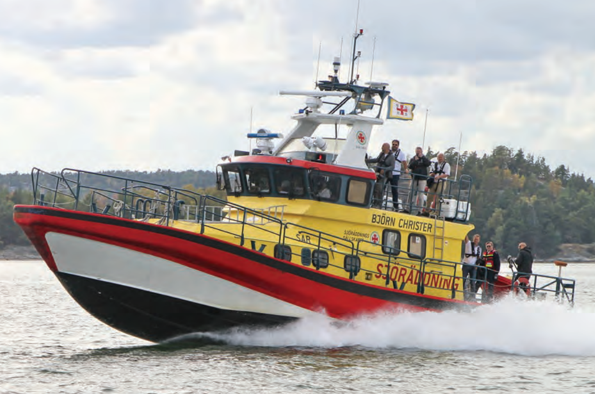
With two times 846 kW at 2,300 rpm via two KaMeWa Rolls-Royce FF 550 jets the vessel accelerates up to 39 knots.
