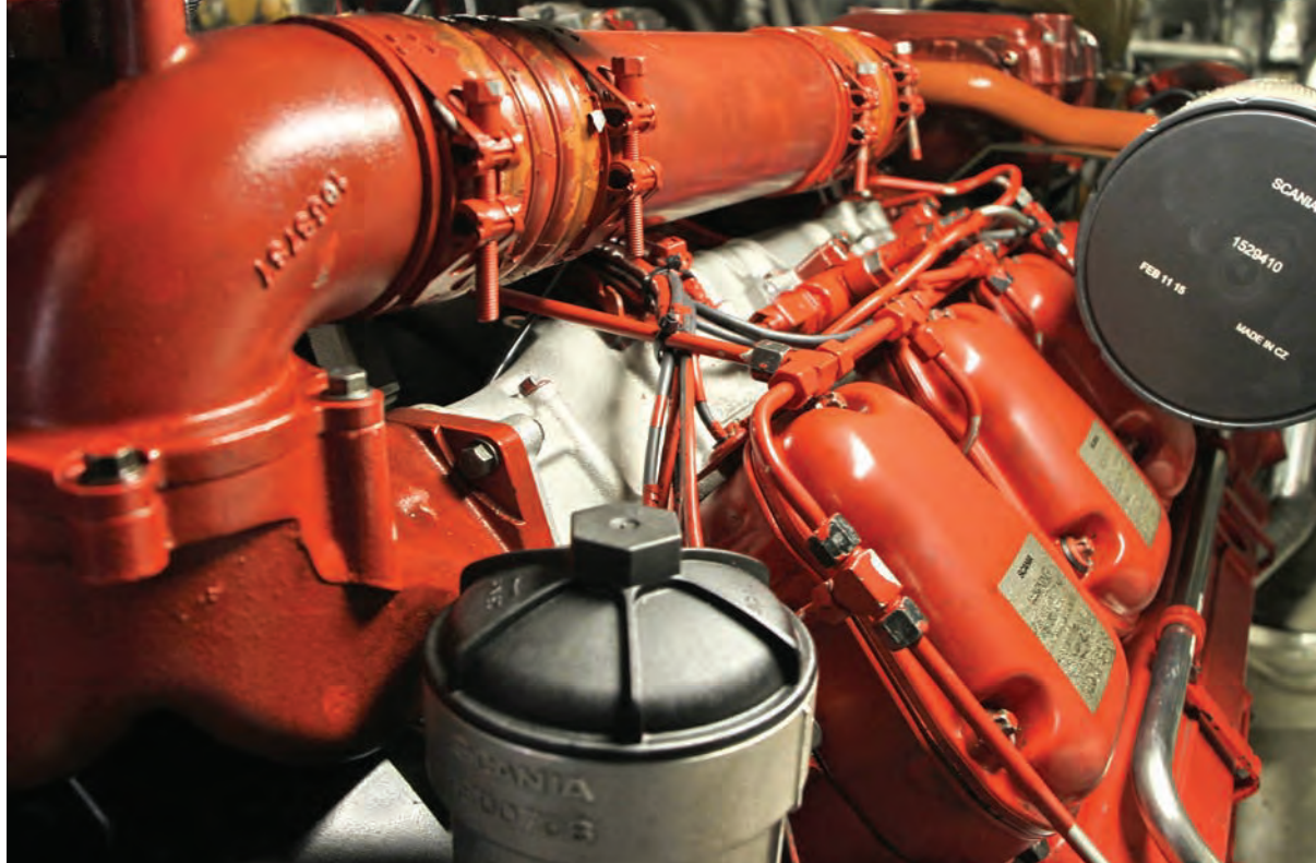
The common rail on the engine.
