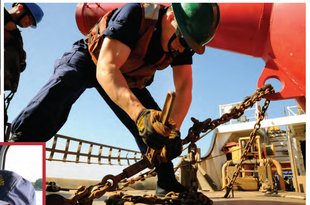
A Coast Guard Cutter Joshua James crewmember chains a buoy to the deck.
