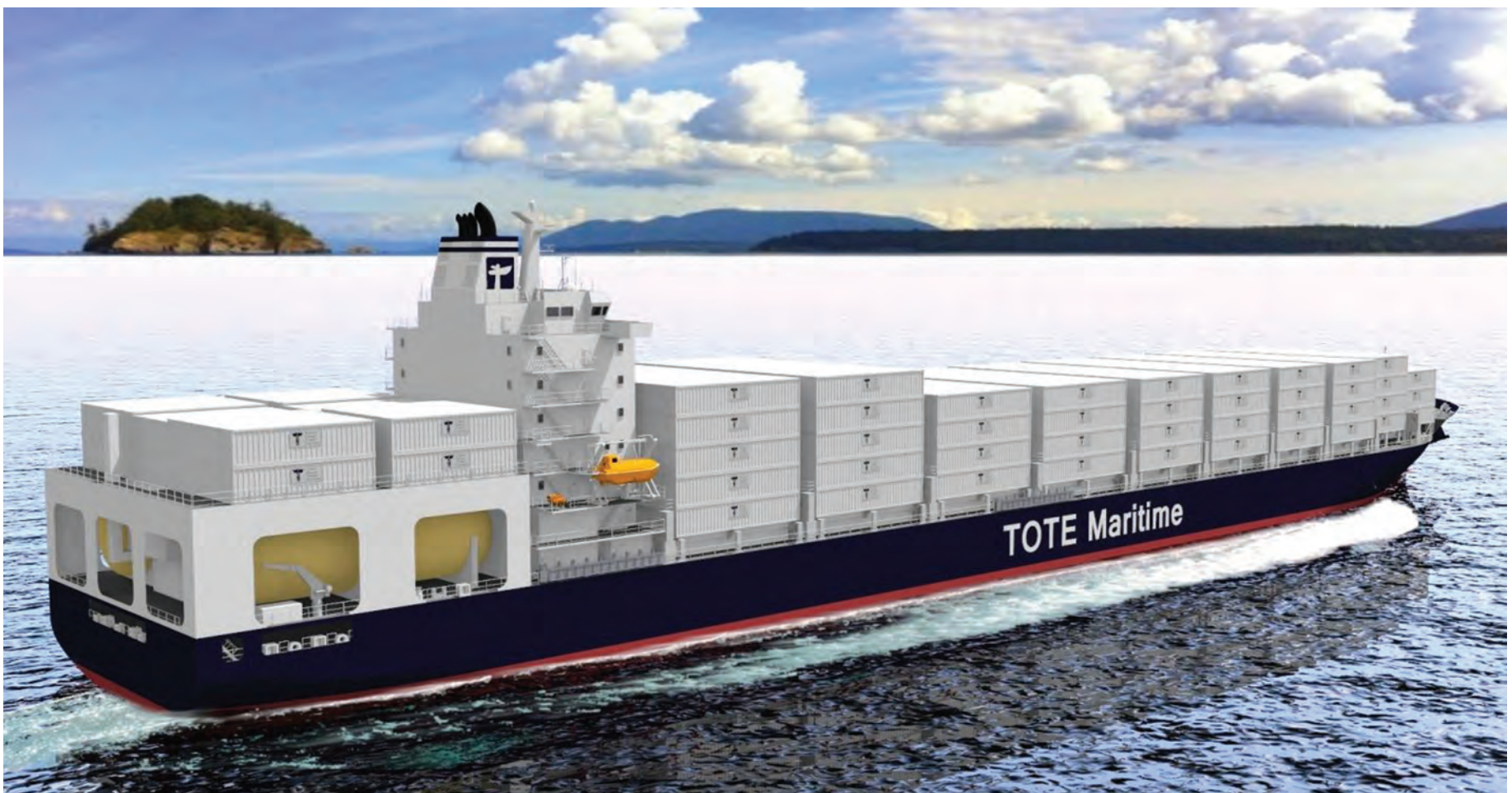
Artist rendering of TOTE's new dual fuel containership, the world's first containership to be powered primarily by LNG. As with other LNG powered designs, fuel tank size and placement will be a major feature.
