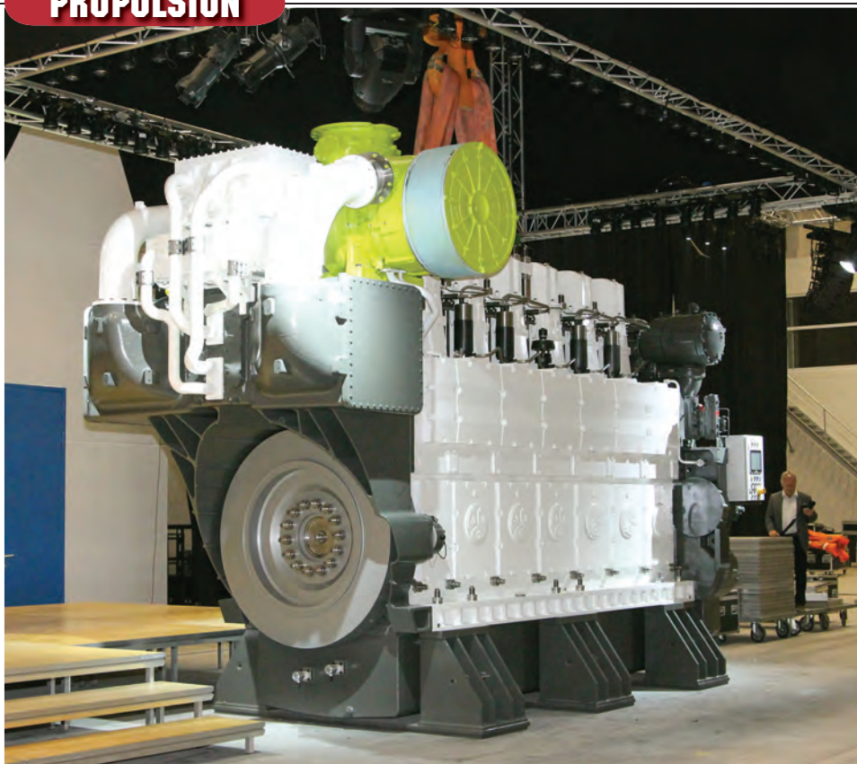
Left The newly developed DL-series comes as a 6 and 8-cylinder in-line version and a 12 and 16-cylinder v-type configuration delivering 650 kW per cylinder.
