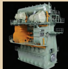
Graphic of the second-generation EGR system (orange) integrated with its host engine
