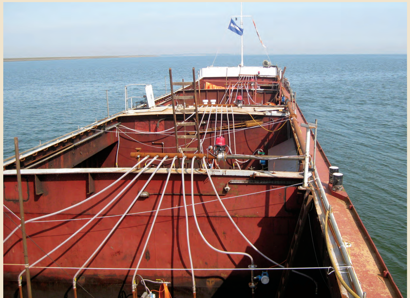
The air supply system of the air cavity ship was reproduced faithfully.
