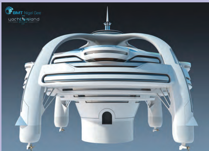
The center section is used to attach the mooring system and houses the main dock. At the base of each leg is an azimuthing thruster providing slow speed propulsion.
