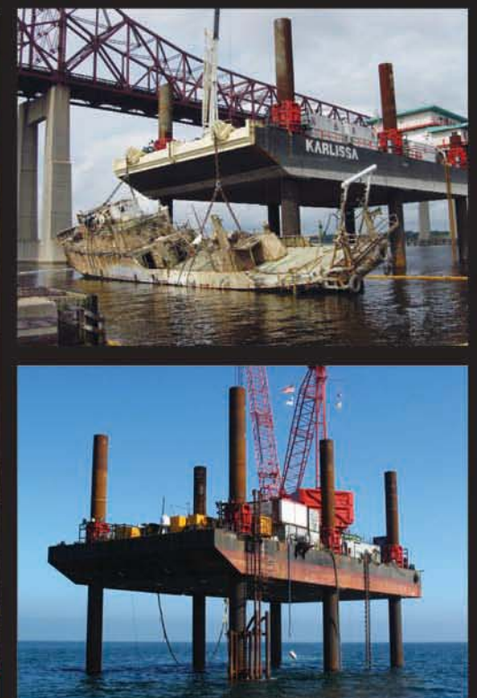
TITAN's jack-up barges, Karlissa A and Karlissa B , used in the wreck removal of the New Carissa in Coos Bay, Oregon.
