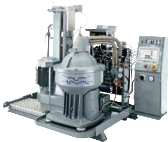
S-separator - Fuel and lube oil cleaning system
