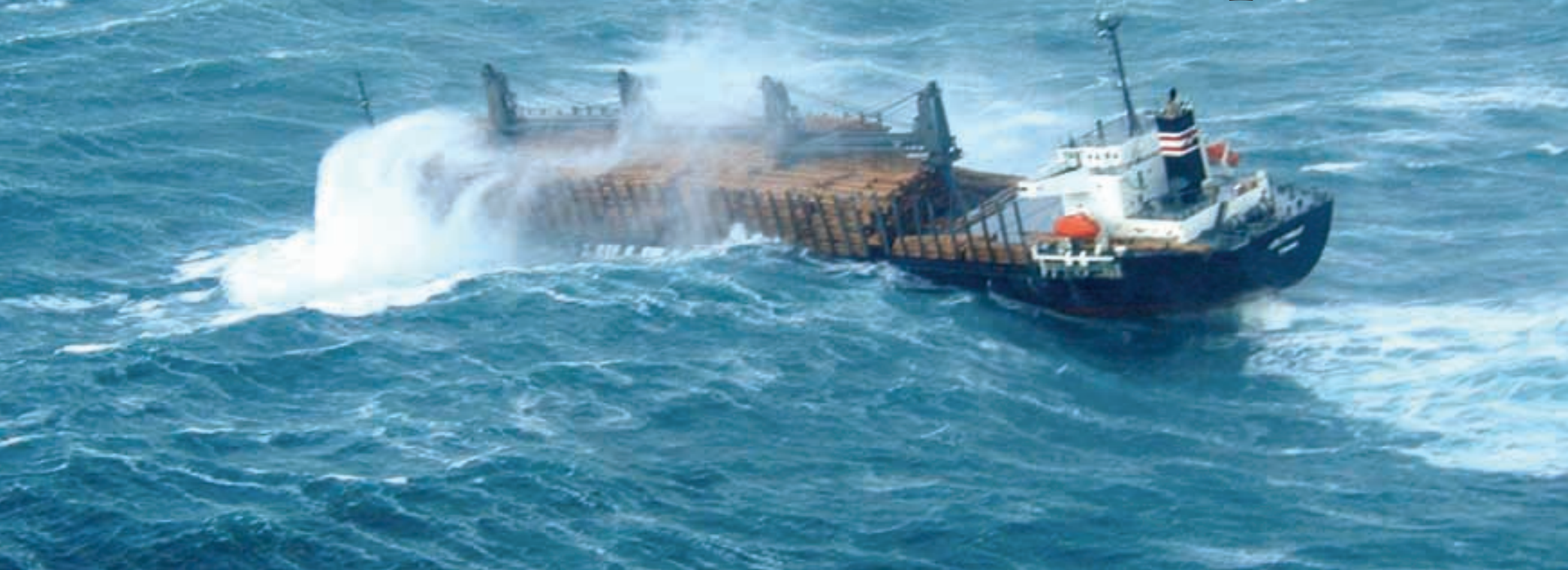
The 551-ft. log ship Forrest in the Bering Sea after losing logs overboard and listing in heavy seas. (USCG photo by Petty Officer Kevin Martin)
