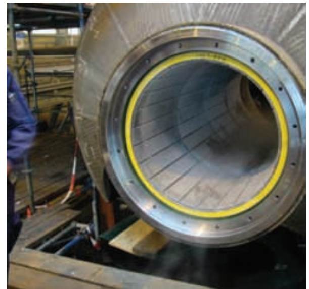
Water lubricated Composite bearings installed in self-propelled ocean going jumbo Cutter Suction Dredger, d'Artagnan, at IHC Holland.
