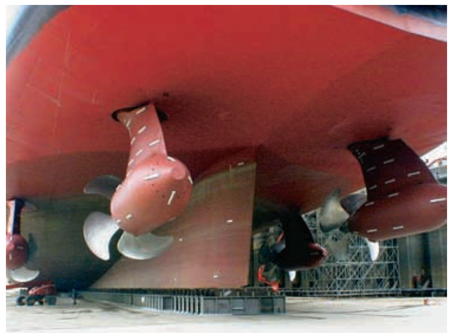
Pods make the ship quieter and virtually free of vibration, even at a speed of 30 knots. Queen Mary 2 has four Rolls-Royce Mermaid pods, two fixed and two azimuthing.
