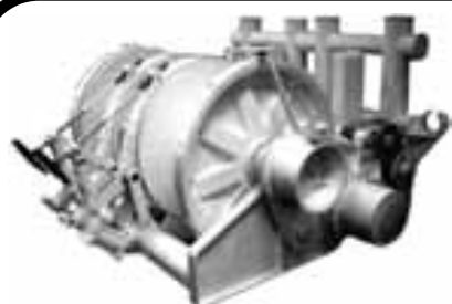
"Burrard heavy duty double drum towing winch as supplied to: Delta Linda, Delta Carey, Delta Deanna, Millennium Falcon, Millennium Star and Millennium Dawn"
