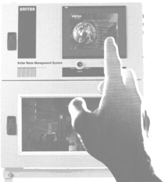
Unitor's new Boiler Water Management System provides continual and precise control of important boiler water and condensate system conditions by automatically monitoring acidity, conductivity, dissolved oxygen and turbidity.
