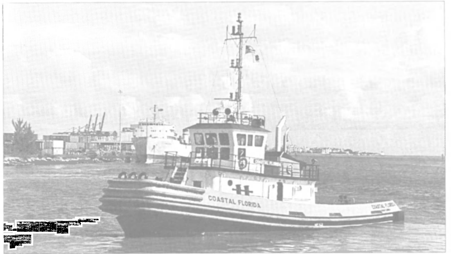
The Coastal Florida, recently delivered by Main Iron Works, is fitted with Ulstein Maritime Z-propeller units which rotate 360 degrees, eliminating the need for rudders.
