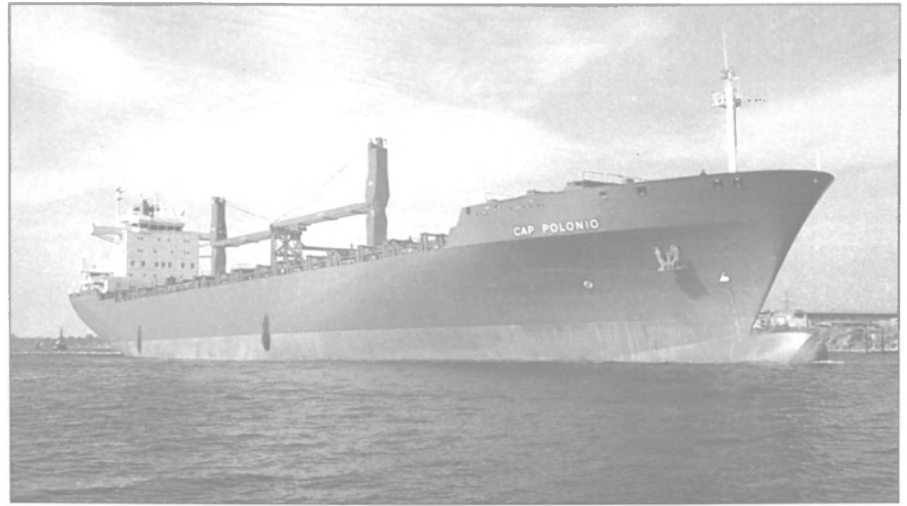
The Cap Polonio is based on Flender Werft's steam-geared containership design "Flender 2000."
