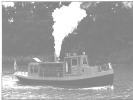
The Bridget 30 tugboat's 30-foot length, 8-foot beam and draft of 2 feet allow her to move easily through the water, achieving speeds up to 10 knots.
