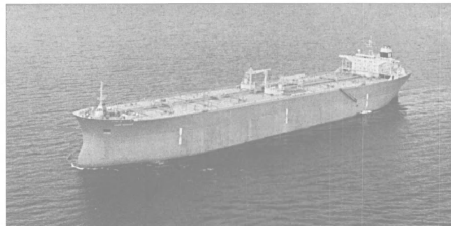
The crude oil carrier Jahre Traveller, from Yugoslav builder Brodosplit, has a liquid cargo capacity of 170,000 m 3 .
