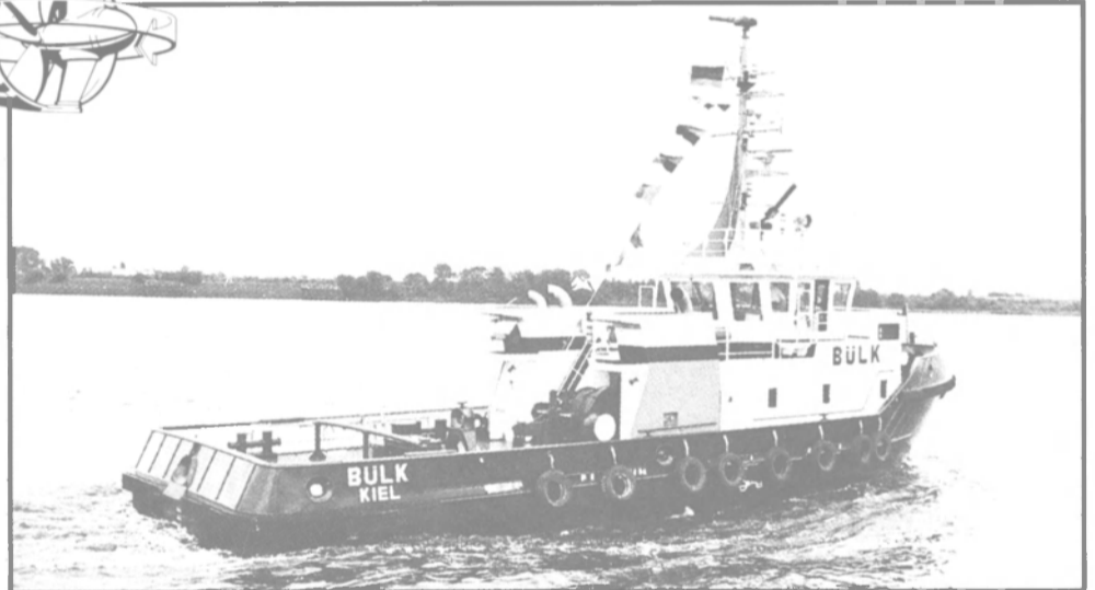
Ice-breaking multi-purpose tug "BULK" with 2 Rudderpropellers, total output 2208 kW, 1 SCHOTTEL Bow Thruster (220 kW) and Anti-Suction-Tunnel A·S·T
