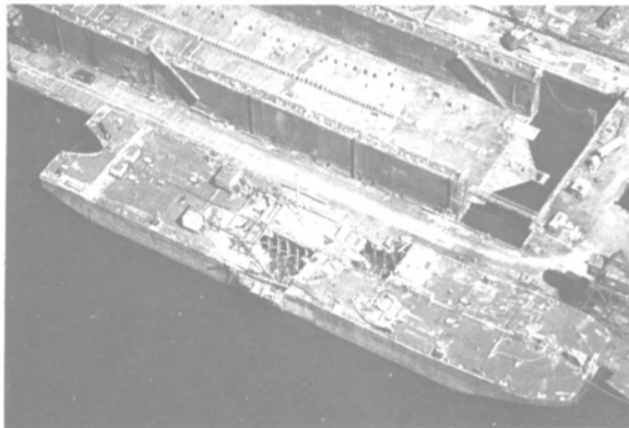
The tank barge Cibro Savannah, which sustained damage after a fire and explosion, is shown in New York Shipyard for repairs.
