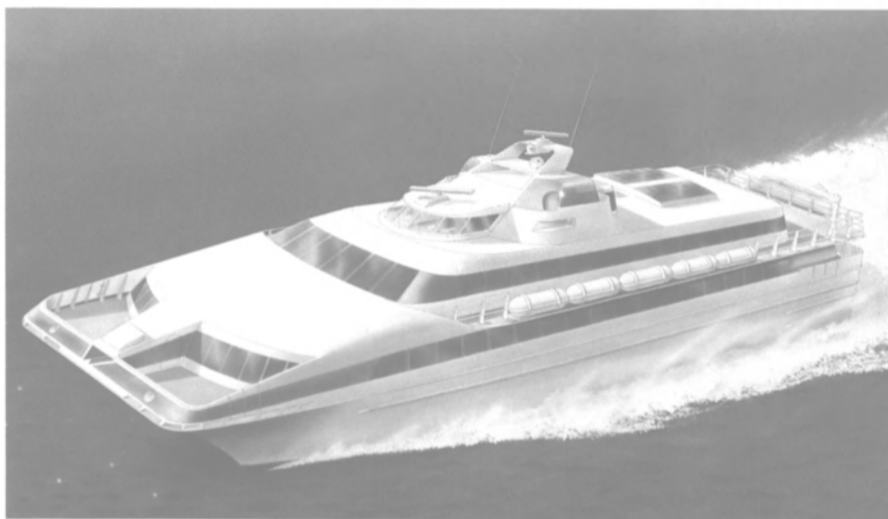
Westamarin's latest high-speed catamaran design, the 4200S (shown above), can cruise at 45 knots.
