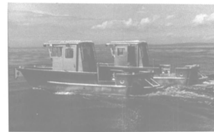
Typical rigid boom deployment and maintenance boats. Munson delivered four of these diesel-powered boats to Valdez oil terminal in Alaska.
