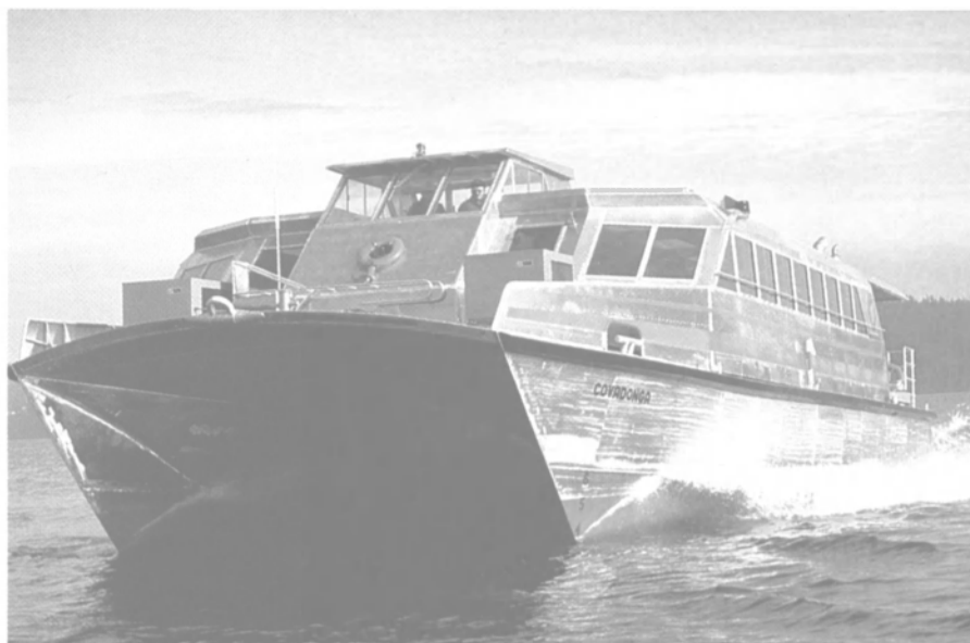
Powered by twin Detroit Diesels, the ferry Covadonga can reach about 28 knots
