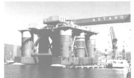
The Friede & Goldman-designed Drillmar I marks the first entry for Astano shipyard into the offshore market.
