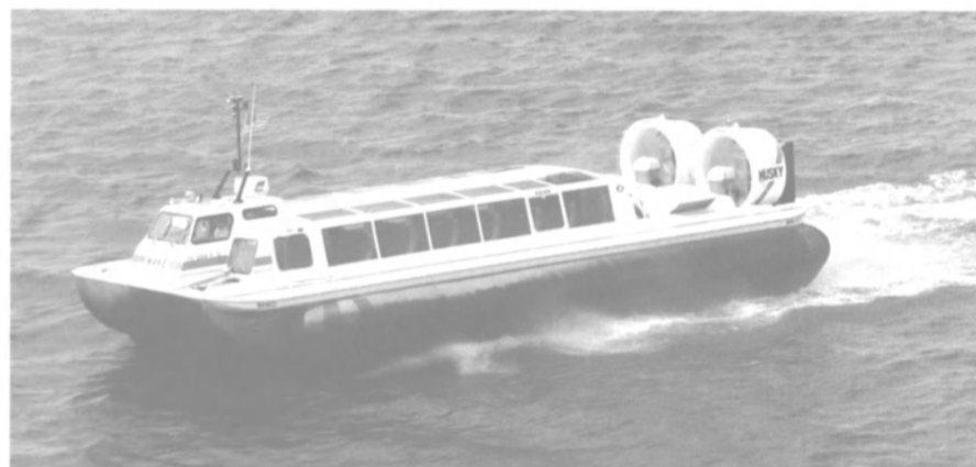
Hover craft consist of a rigid hull and superstructure supported on a cushion of air provided by internal centrifugal fans and contained under the craft by a flexible loop and segmented, ducted skirt. Propulsion is provided by one or more ducted propellers which are diesel driven.
