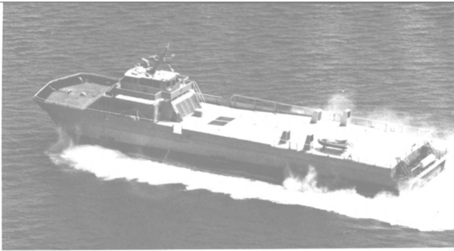
The U.S. Navy SES-200, to be powered by twin MTU 16V396TB94 marine diesel engines and KaMeWa waterjets.
