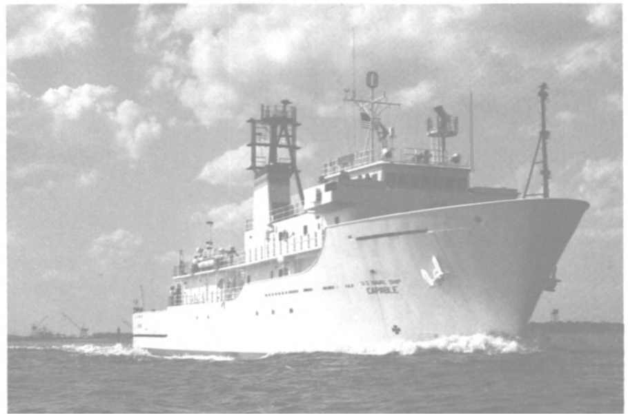
The 224-foot Capable is powered by four Caterpillar/Kato 600-kw generators driving two General Electric motors.
