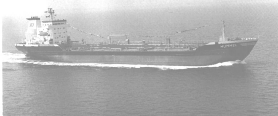
The double-skin chemical tanker Hummel, built by West German-based Lindenau Shipyard for Carl Buttner Shipping Company, is powered by a single Krupp MaK engine to speeds of 14 knots.
