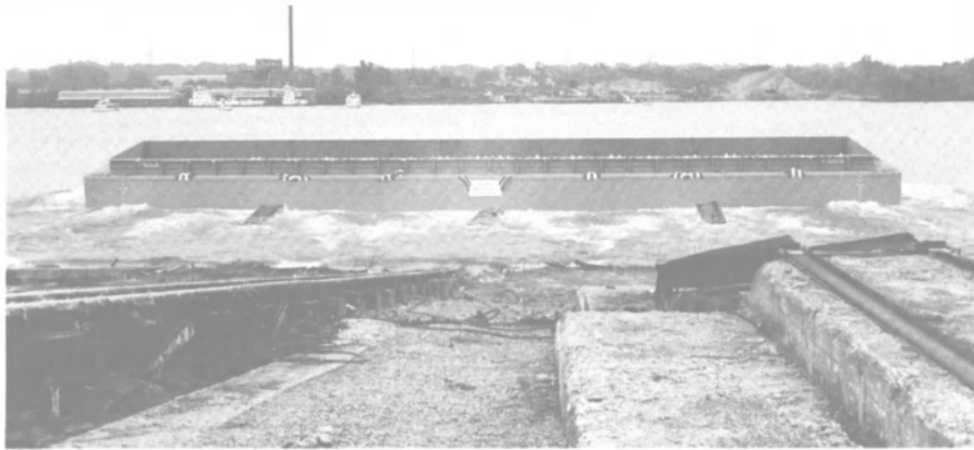
The jumbo hopper barge, shown above after launching by Jeffboat, is the first barge built since the yard reopened for new construction.
