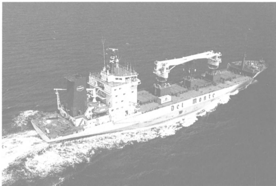
The first of four 370,000-cubic-foot reefers being built by the Sevilla shipyard of AESA, the Del Monte Planter will be powered by a single MAN B&W-AESA 6L60MC engine. Eight other Del Monte reefers being built by the yard will feature the same engine.
