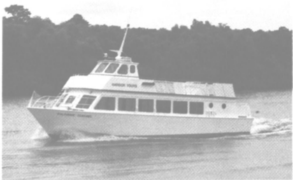
The Cummins-powered Baltimore Sentinel is 63 feet in length, with a 20-foot beam, and a 3-foot draft.
