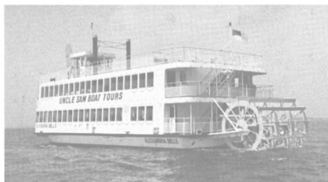
ALEXANDRIA BELLE July 1988 87' x 32' x 8' Steel Dinner Boat Owner: Uncle Sam Boat Tours Thousand Islands, NY
