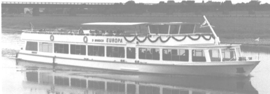
The M.S. Europa, seen here on the Weser River in West Germany, is the first passenger vessel to be propelled by Schottel Pump-Jets.
