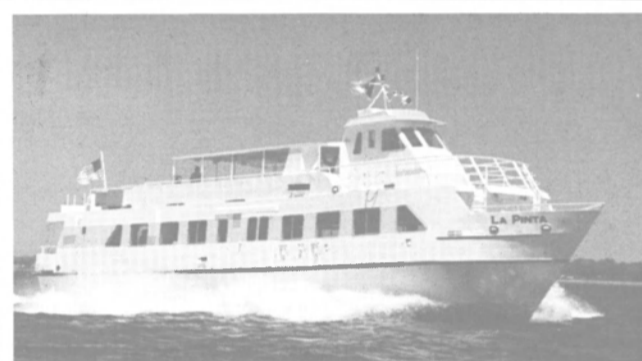
LA PINTA June 1988 92' x 22' x 5' Aluminum Passenger Ferry Owner: Puerto Rico Ports Authority San Juan, Puerto Rico
