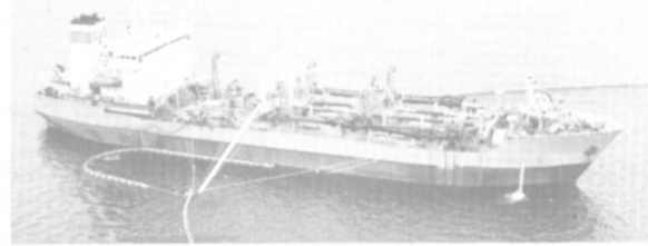
Multipurpose Vaydaghubsky can operate as oil recovery vessel, dredge or fireboat.
