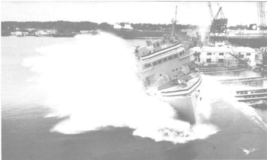
The 224-foot-long MCM-3 Sentry is the second mine countermeasure ship of this new class to be launched at Peterson Builders, Sturgeon Bay, Wisc.
