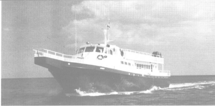
The Spirit, shown above, was converted from a 96-foot aluminum crewboat to a 149-passenger whale watch/excursion vessel.
