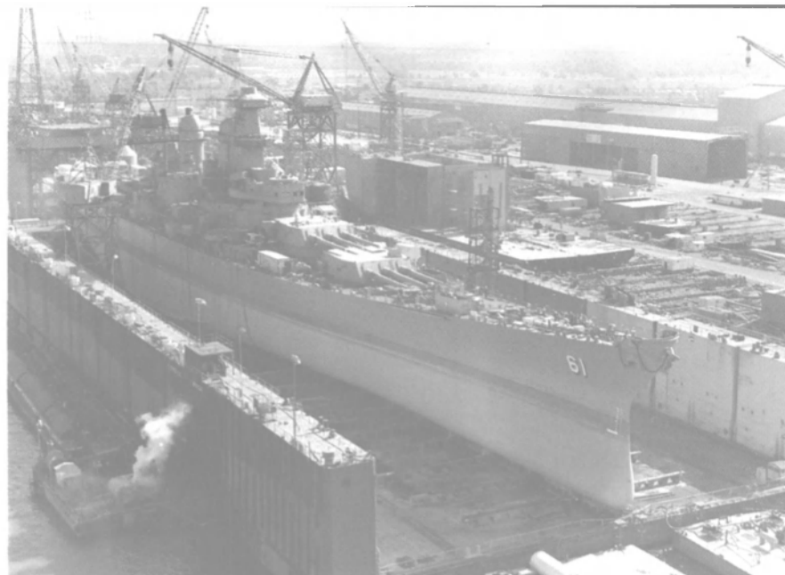
Avondale's 81,000-ton floating drydock (above) used to reactivate the Iowa (BB 61) will also be used for work on the Wisconsin (BB 64).
