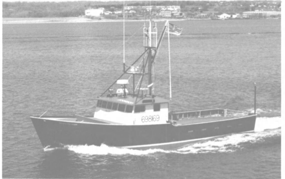
The Gladding-Hearn Sally & Katherine features a Caterpillar 3408 DITA marine engine rated at 402 hp at 1,800 rpm.
