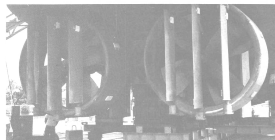
The Towmaster Rudder System being installed on the harbor tug Esperanza.
