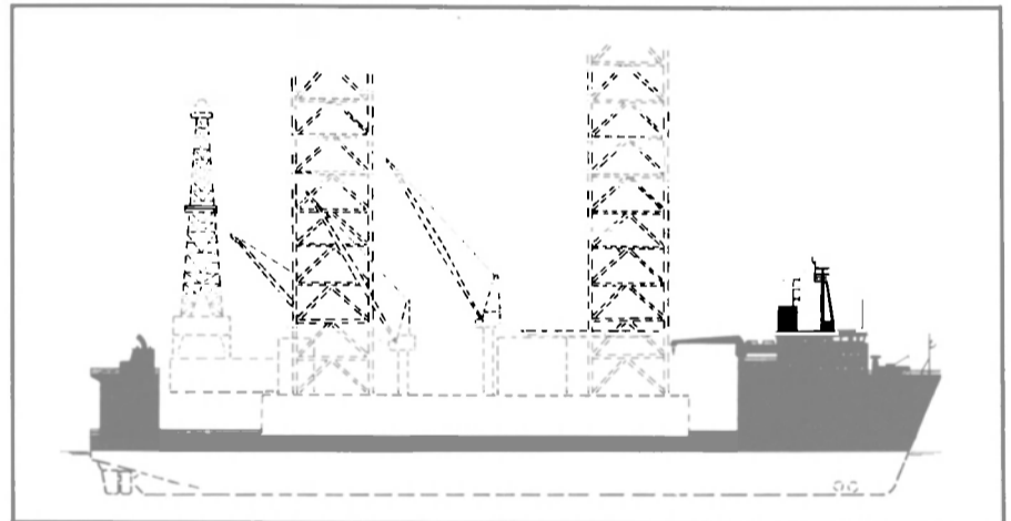
Drawing of specialized vessel being built for the Soviet Union by the Wartsila Turku Shipyard, which will transport floating oil drilling rigs.
