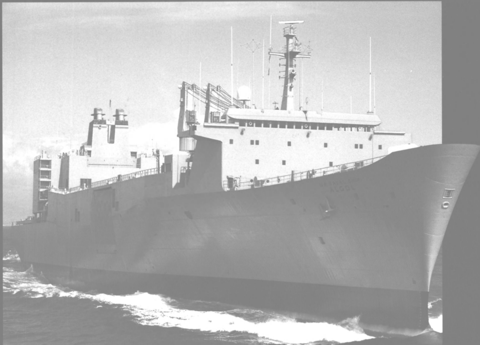
USNS Algol (T-AKR—287), first of three Fast Logistic Support Ships after conversion at NASSCO for the U.S. Navy, underway at more than 33 knots.
