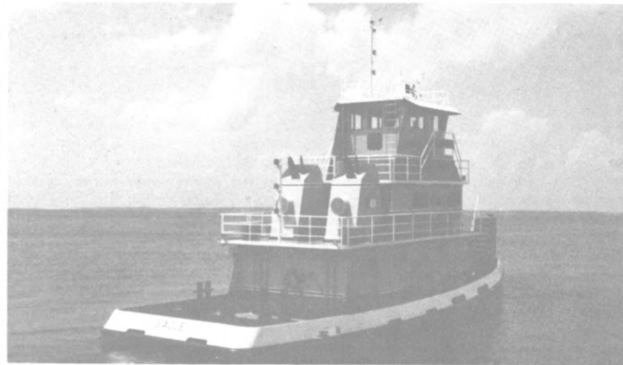
Eastern's new towboat Eagle is powered by two Detroit Diesel 12V-149N engines.
