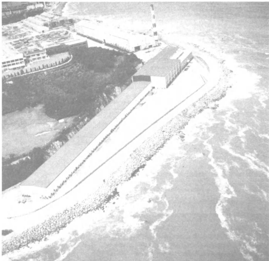
Aerial view of HMRI facility near Hyundai's shipyard and engine factory in Ulsan overlooking Korea's East Sea. Long extension at left houses 690-foot-long towing tank.
