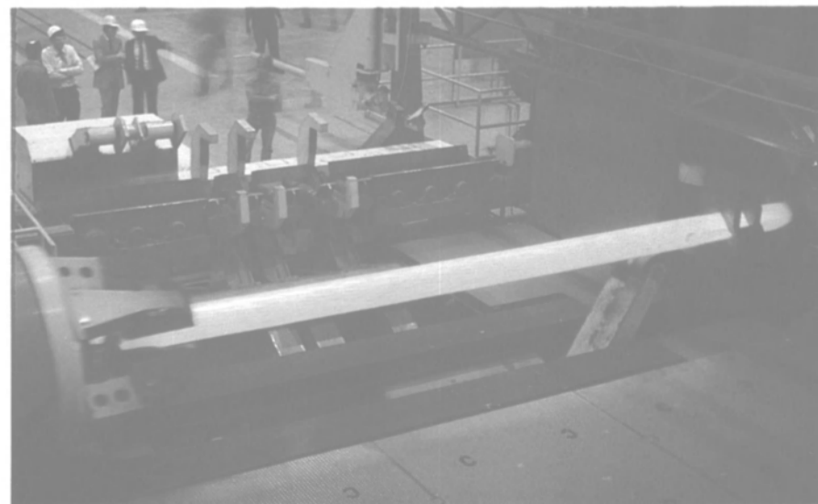
Precision forging machine in operation at Armco's expanded Baltimore Works.
