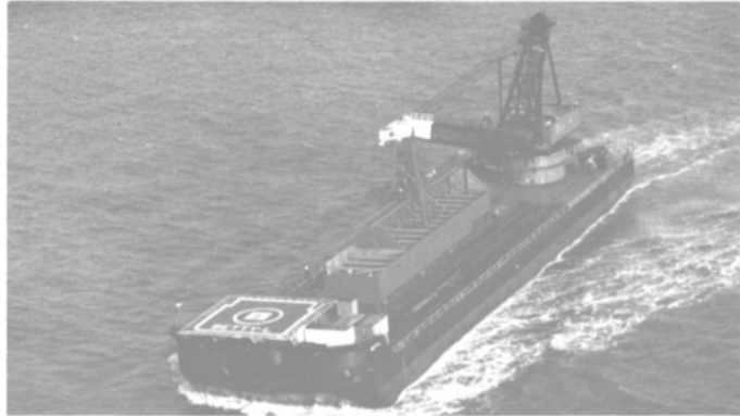
400' x 98' x 25' heavy construction barge with 500 ton capacity crane and 4000 cubic yard gravel bin.
