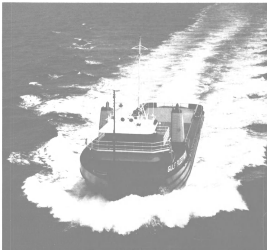
Towing/supply vessel Gulf Fleet No. 41 is New Orleans-based company's 101st vessel. Built by Quality Shipyards, she is powered by General Motors EMD main engines.
