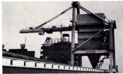
Bulk Unloaders —One of the world's largest Alumina unloaders, designed by PACECO with dust enclosure over hopper and sealed clamshell bucket. Handles 1000 Long Tons per hour with minimum loss of material.
