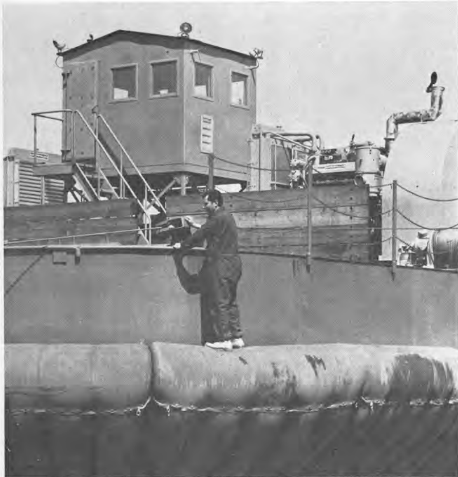
ACT-100 is on all-steel barge-type hull with a flexible containment skirt around its perimeter. Here air-lifted, the hull rises four feet off the ground.
