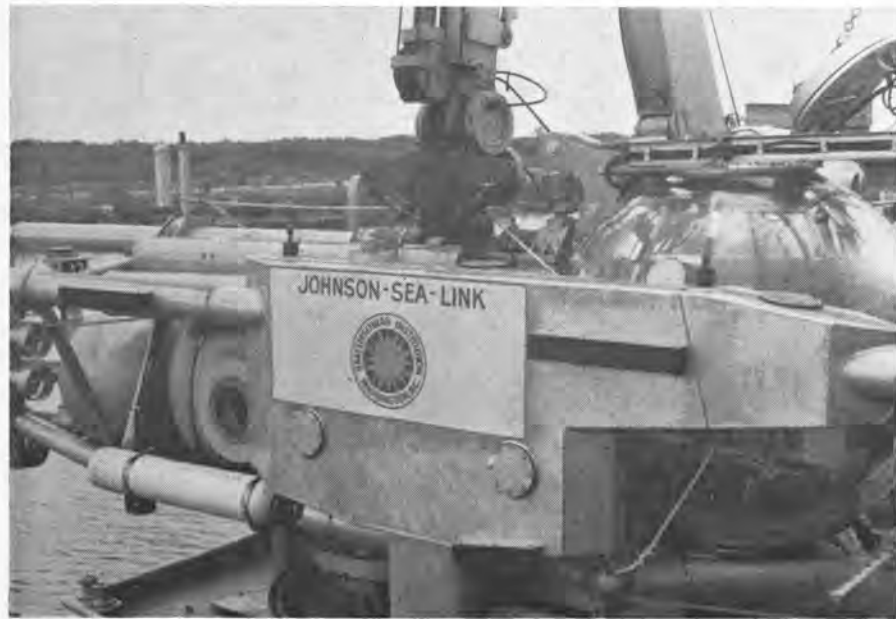
Johnson-Sea-Link Smithsonian submersible. Six-foot diameter acrylic sphere accommodates two men in control compartment. Three-man diving chamber is behind. Craft can maneuver in any direction at depths up to 1,000 feet. A special hydraulic crane handles the vessel on or off support ship Sea Diver.
