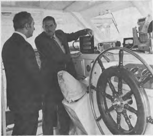
Morton J. Howard, Sperry Marine Systems Division, points to the speed and distance reading of the new Doppler Speed Log in the pilothouse of the demonstration vessel.
