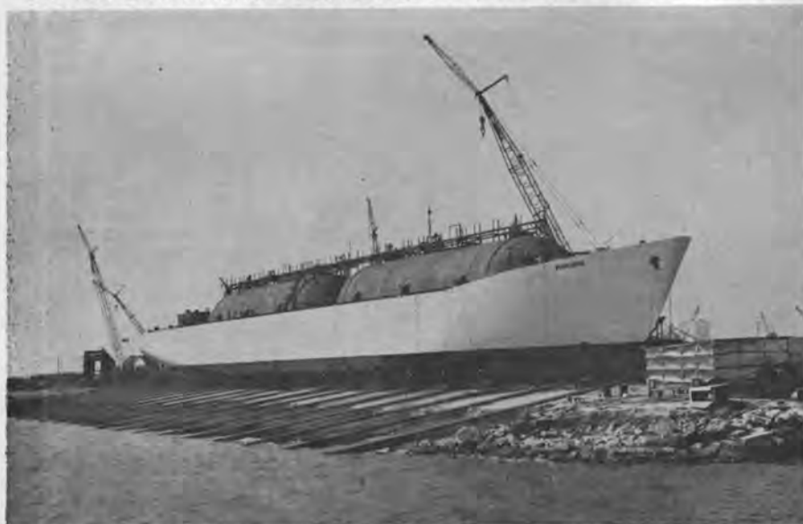
The Ponciana, built with a modified ship's bow and deep stern notch for push towing, carries what is believed to be the largest cylindrical tanks in barge transportation.
