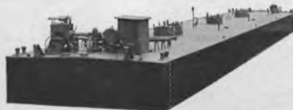
Double square-end, single skin tank barge
