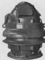
WESTINGHOUSE MAIN CARGO PUMP MOTORS
