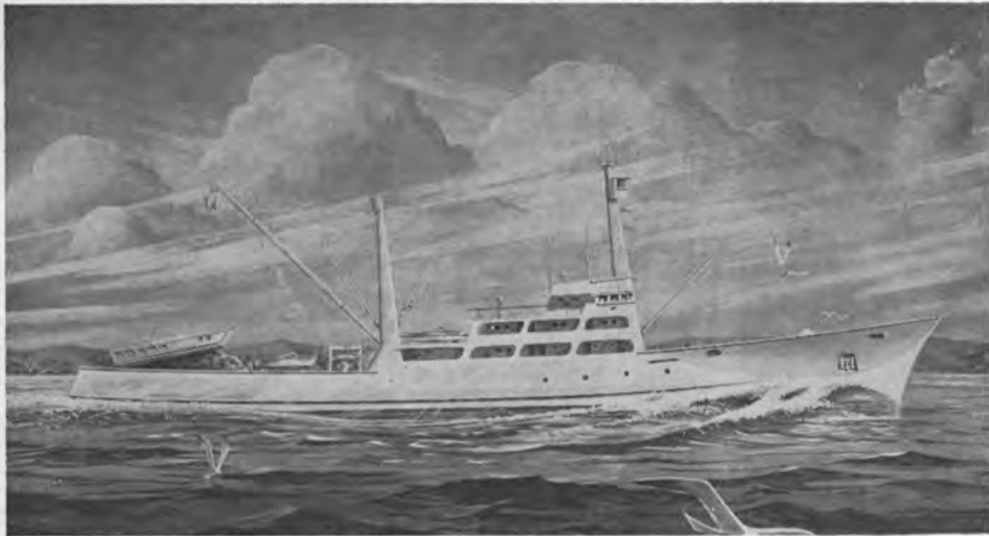
Artist's conception of the 3,500-ton tuna seiner Margaret L. which displays a yacht-like profile. The crew's nest, 92 feet above the waterline, will be reached by an elevator installed in the hollow mainmast rising from the bridge structure.
