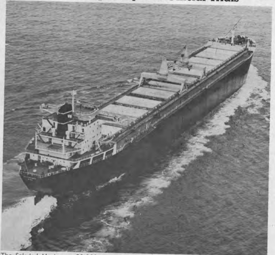
The Soledad Maria, an 80,000-dwt bulk carrier built by Astilleros Espanoles S.A., is shown in the Bay of Cadiz during the official sea trials. The ship was designed with the maximum dimensions for transiting the Panama Canal.
