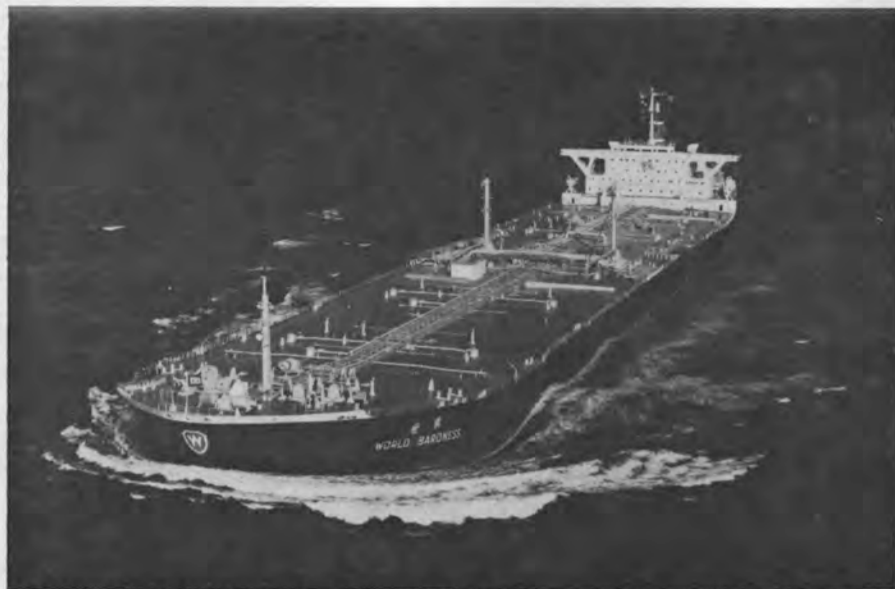
228,825-DWT TANKER: Hitachi Zosen's Sakai Shipyard recently delivered the 228,825-dwt tanker World Baroness to Liberian Shield Transports Inc. This is the third vessel of the 230,000-ton type series. The first vessel of this series, Eiko Maru , was completed in April 1971, and the second, Sanko Lake , was completed in June 1971. The new tanker, measuring approximately 1,001 feet by 167 feet by 85 feet, is powered by a steam turbine with a maximum output of 33,000 hp producing a speed of 16.2 knots. The main turbine and boilers are controlled from the wheelhouse, and the engine control room and watching of principal auxiliary machinery is centralized. The tank arrangement and cargo system is designed for the carriage of different cargoes of crude oil.
