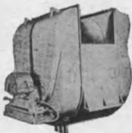
WESTINGHOUSE MAIN GENERATOR STATOR
