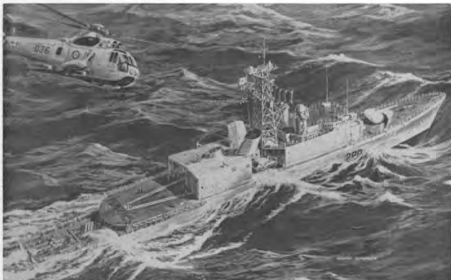
Artist's conception of helicopter-equipped Canadian destroyers for which Marine Industries has been selected as lead yard. These ships will have gas-turbine propulsion.
