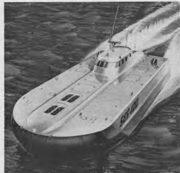
Artist's conception of 100-ton SES proposed by Bell Aerosystems. This testcraft measures approximately 72 feet long and has a width of 33 feet. It is being designed for speeds in excess of 80 knots.
