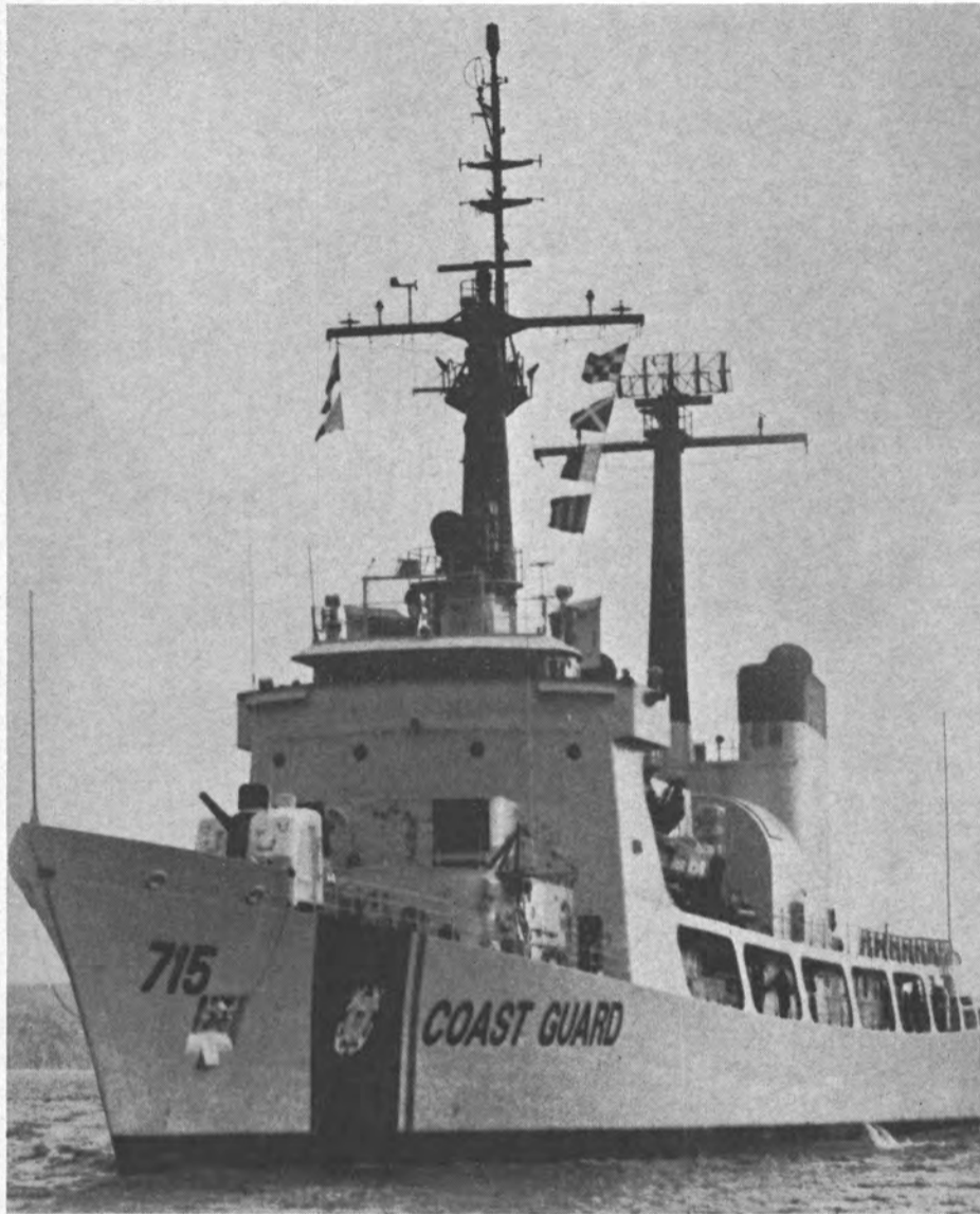
USCGC HAMILTON, WHEC-715—one of nine similar vessels designed by the U.S. Coast Guard. All of these ships, built by Avondale Shipyards, Inc., have York air conditioning equipment. Three York hermetic cooling plants provide crew comfort—and cooling for computers and related equipment. Two smaller York machines are used in ship stores facilities.
