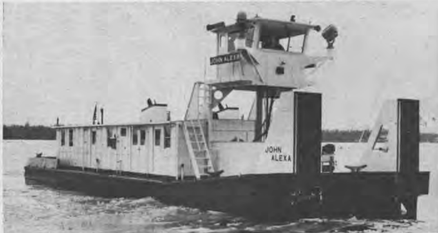
The retractable pilothouse on the John Alexa gives the pilot a 23-foot eye level when raised and only a 15-foot overall height when retracted.
