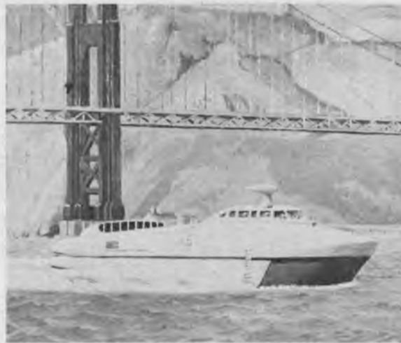
Artist's rendering of SES proposed by Aerojet-General. The design calls for a vessel 80 feet long and 37 feet wide. When built, construction would be at Tacoma Boat Building Company, with testing on Puget Sound.
