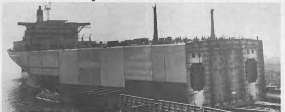
Stern section of 210,000-dwt tanker is launched at the Amsterdam yard of NDSM.
