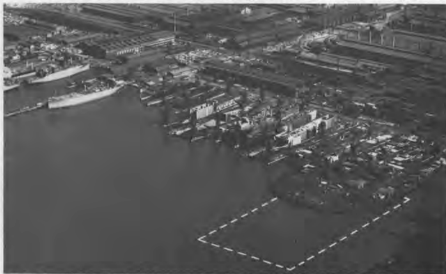
Aerial view of Bethlehem Steel Company's Sparrows Point, Md. shipyard with steel mill in background. Broken white line indicates location and size of new shipbuilding basin for constructing ships of 200,000 dwt or more and over 1,000 feet long.
