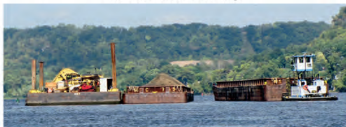
136 x 30 x 12 Ft Spud Deck, 150 x 35 x 8 Ft Barge & 200 Ft x 35 Ft x 10 Ft 6 In. Barge
