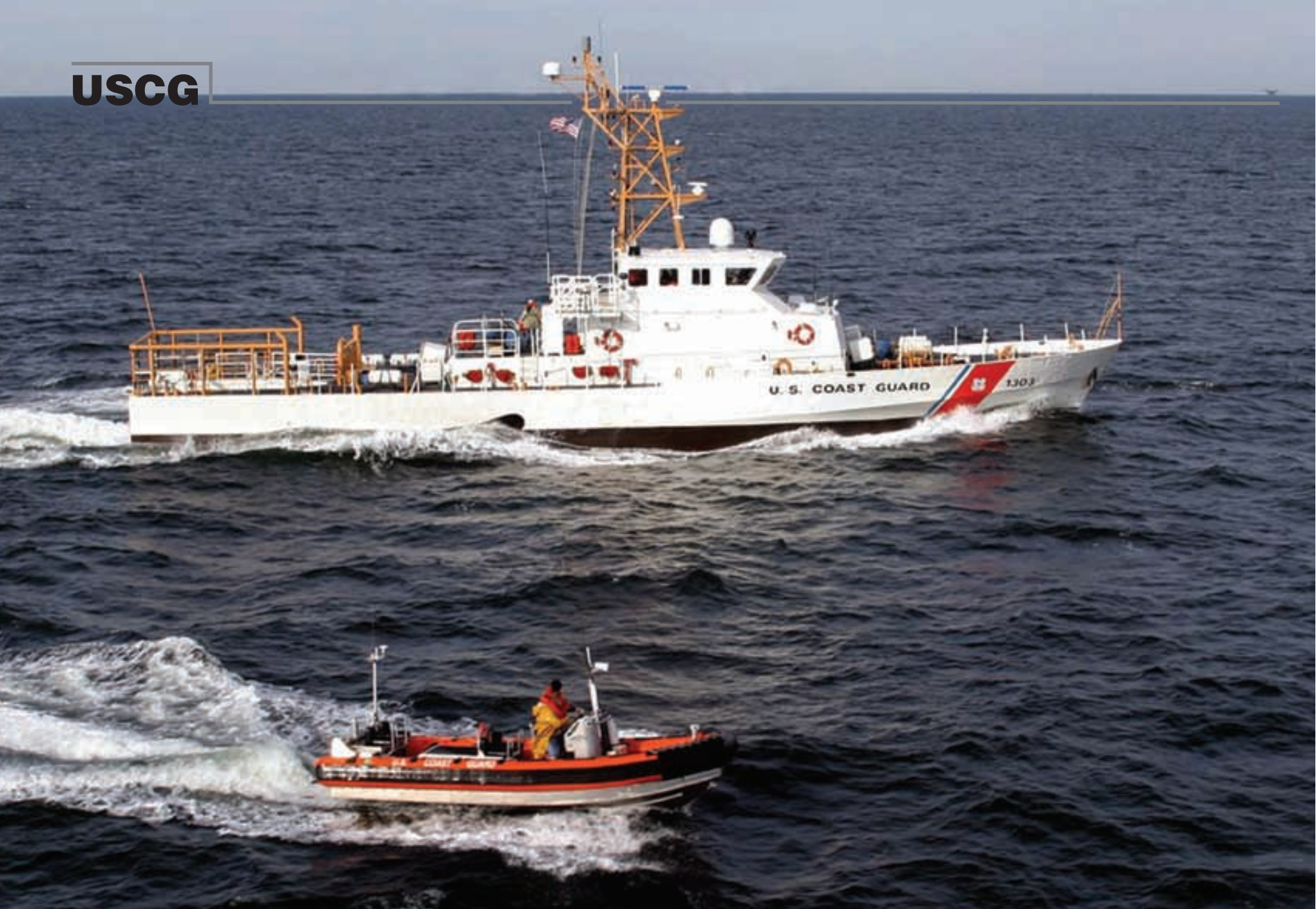
The 123-ft. Coast Guard patrol boat Matagorda on sea trials with her RIB deployed.
