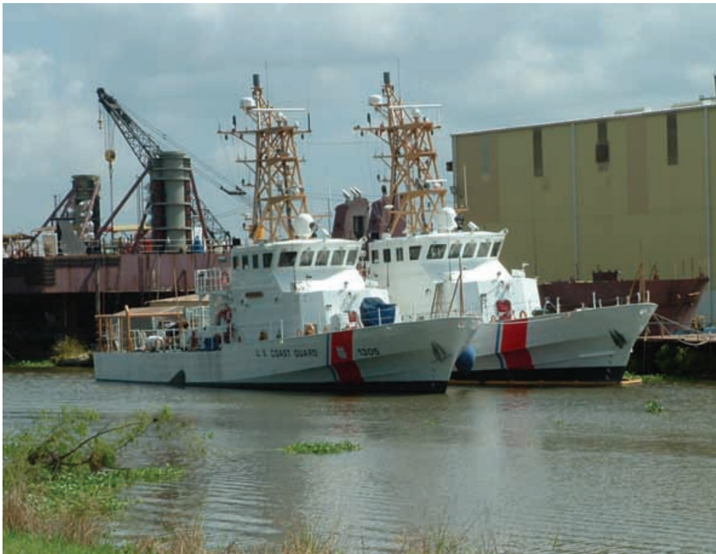
A pair of the Island Class patrol boats undergoing final outfitting at Bollinger Shipyards, Lockport, La. A total of eight of these vessels were upgraded to carry the SRP in a 13-ft. addition to the stern lengthening the vessels to 123 ft.
