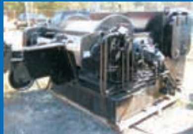
RESEARCH & SPECIALTY WINCHES -- This hydrographic is but one of several types aboard NOAA's FRV-40 Oscar Dyson
