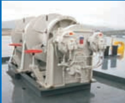
TOWING WINCHES -- recent order for M/V Saturn matches winches supplied to Western Towboat
