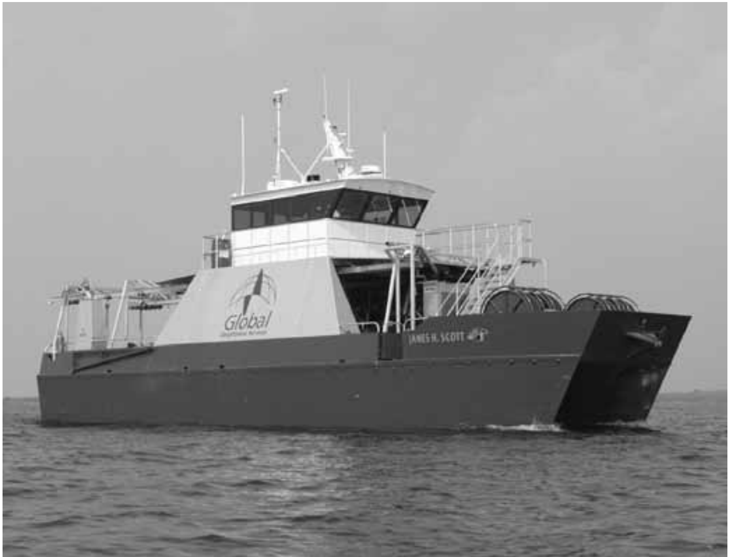
The James H. Scott on sea trials near the builder's shipyard. The catamaran design makes for an inherently stable vessel.
