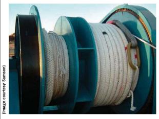
A custom-engineered tapered high-performance synthetic winch line used on the Enfield riser column installation in 2007.
