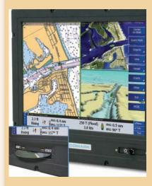
Comark Corp. announced the availability of a front access DVD/USB option for the MDU19PC marine panel computer, to allows for quick data or program updates at the console, without having to remove the display from the panel, load software on a remote computer, or use portable drives. The option is specifically targeted at ECDIS and ECDIS-N applications that require periodic data updates to remain compliant
