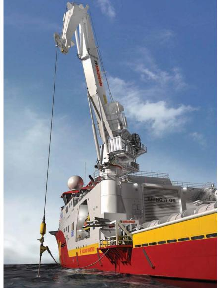
The MacGregor ultra-deepwater lifting system uses new multi-component fibre ropes that weigh nothing in water.
