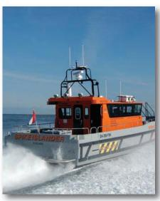
Ultra Dynamics supplied three sets of twin UltraJet UJ377 Waterjet installations to South Boats for their New Mk II GRP 43/12m WFSV RRV Catamarans RRV Audrey, Offshore Response 1, and Spike Islander. The GRP catamarans have all been tailored to meet specific code and operational requirements of Wind Farm operations operators Turbine Transfers (Holyhead Towing) and Offshore Wind Power Marine Services:Limited (OWPMS) and Waddentaxi in the Netherlands respectively.
