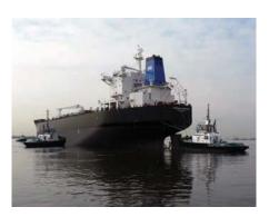
pleted by 2011. The 46,000 dwt vessel was floated off of its blocks and was transferred by tug from the Building Dock to the Outfitting Dock. When completed, the 600 ft. Overseas Martinez will be sold to American Shipping Company and bareboat chartered to OSG America.
