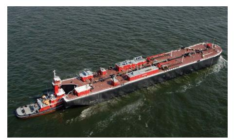
trials. Returning to full service as an ATB asphalt capable tank barge, the barge measures 483 x 80 x 36.2 ft. without the tug coupled into the notch. At the same time that the Barge B. No 235 was taken out of service, the accompanying tug, J. George Betz, was delivered to the Bollinger Algiers facility to install the In-
