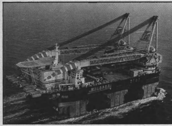
Semisubmersible crane vessel Micoperi 7000 en route to a deep water job. The vessel features twin AmClyde 7,000-metric-ton cranes.
