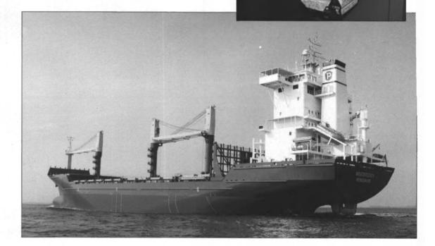
Hanjin Heavy Industries Yard: **Nedlloyd River Plate** Ship: Type: **Container Carrier Leonhardt & Brumberg** Owner: **Designer:** HHIC Length (o.a.): 551 ft. (168 m) Length (b.p.): 518 ft. (158 m) Breadth, molded: 89 ft. (27.2 m)
