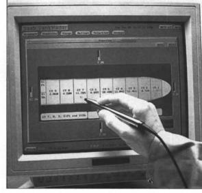
Saab has introduced a third generation of its TankRadar level gauging system, which uses a light pen to activate the system's various func-
