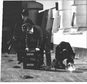
Unitor introduced a compact, lightweight, mulipurpose electric welding unit for shipboard use. Developed with Lincoln Electric, the UWI-350MP s designed to cover all shipboard arc welding and utting requirements — but for operators who only require conventional coated electrode weldng, comes in a basic form with a comprehensive ist of "add-on" features.
