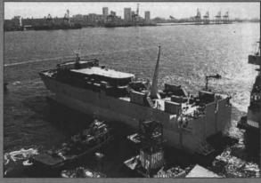
Kawasaki Heavy Industries Inc. launched a wave-piercing catamaran aluminum high speed ar ferry, type Kawasaki Jet Piercer AMD 1500 Mark II for joint owners Maritime Credit Corporation of Japan, Tokyo and Kyushi Ferry Boat Co., Ltd., Yawatahama, Ehime Prefecture. The vessel is based on a design from Advanced
