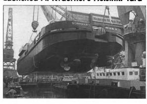
The river icebreaker Rothelstein, for the Osterreichische Donaukraftwerke AG, Austria, has been launched at Kvaerner Masa-Yards' Helsinki New Shipyard. The vessel, to be delivered in spring 1995, will operate in assisting river traffic and break ice formations at the ower stations in the river Danube.
