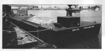
Length Beam 180'0" Depth of Mid-Body 14'0" 128'0" Hopper Length Level Hopper Volume DWT @ d = 10.22 ft. 1421 cu. yd. 1615 L.T. Rake Lengths F. & A. 26'0" Twin Skegs Stern & Fwd. Rake Decks Stepped up 2'0" Engine GM 671
