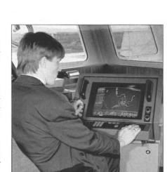
The navigation system NCIS 1800 from Krupp Atlas Elektronik offers the user versatile decisionmaking aids for navigation. It performs monitoring and advisory functions, ensuring high operational safety of the ship.
