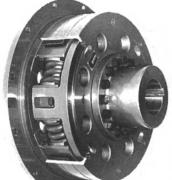
LO-REZ helical steel-spring couplings, with their low, constant and accurately-controlled torsional stiffness factors, provide excellent torsional characteristics for geared marine reciprocating propulsion systems, engine and reciprocating compressor drives of many varieties, locomotive drives, etc.
