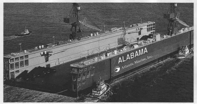
The ALABAMA has a lifting capacity of 250,000 DWT or 50,000 tons displacement. Normal maximum draft over six-foot keel blocks is 32 feet.
