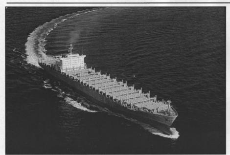
The 4,469-TEU containership Bunga Pelangi, one of the largest in the world, is powered by a single Hyundai-MAN B&W 10K 90MC main engine.
