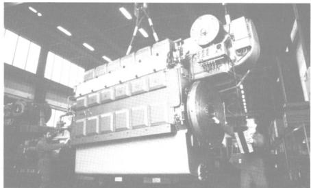
The 28/32A engine type has 280-mm and with 12 and 16 cylinders in V-form. The bore/320-mm stroke. The engine type is output is 1,320-3,520 kw (1,800-4,800 bhp) available with 6, 8, and 9 cylinders in-line
