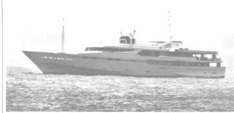
The 201-foot, Italian-built II Vagabondo is equipped with 12-cylinder Deutz MWM 628 Series engines. The 1,050-ton passenger boat can reach speeds of 18 knots.
