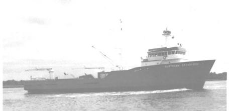
The Northern Enterprise is shown above after conversion. The crabber/processor is powered by two EMD 12-567-BC diesels with Falk 2.98:1 reverse/reduction gears.
