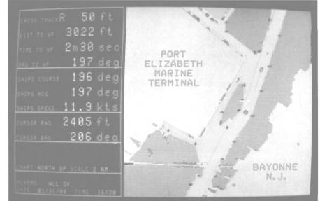
By combining the electronic charts with radar images, the new system gives operators electronic computer generated charts, precise position fixes and radar targets, all on a single clear display.
