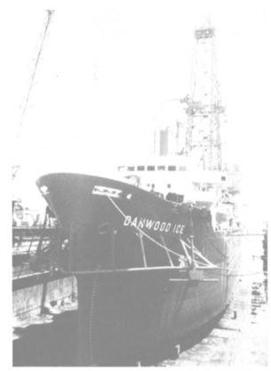
J.L. Offshore Drilling Inc.'s drillship 'Danwood Ice' (pictured above) was recently put in at Hongkong United Dockyards for special survey and overhaul. During her 34-day stay at HUD, extensive steelwork renewals and tank coating was carried out, as well as main and auxiliary machinery overhauls and surveys. The vessel was also drydocked during the period and underwent hull blasting and coating along with routine underwater work.
