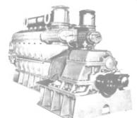
ENGINE: GM 12-567A-8½X10-VEE type-2-cycle-747 RPM-electric starting-serial Nos. 1041 & 1060. GEAR: Falk Air Flex-reverse & reduction-2.48:1 forward-2.52:1 reverse.
