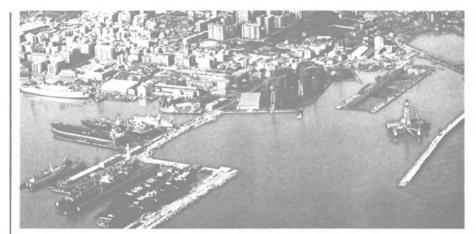
Aerial view of Cantieri Navali Rinunite shipbuilding and repair yard in Palermo, Sicily. New 400,000-dwt drydock is located in basin at right (with drilling rig). In center is small graving dock, and to the left of the aircraft carrier are two other drydocks. Yard currently has conversion/repair orders of \$7 million.
