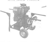
ENGINE: Mfg. by V.M.—air-cooled model HR192A—13.5 HP—3000 RPM—rope start (crank optional). PUMP: Hale—cast iron—3"—N.P.T.—hand priming—weight 410 lbs. Carrier mounted with 2 pneumatic tires for easy handling or 2-man hand carry. Ideal for oil barge, tankers, dockside, etc use.
