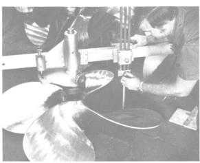
Michigan's Work-Horse<sup>TM</sup> is a tough 4-blade propeller with heavy cross-sections and heavy-duty leading edges designed to give you smoother operation than the 3-blade wheel it replaces. It is cast and available in three very strong materials: Michalloy K bronze and Ni-Bral through 30' dia., and CF 3 mod Stainless Steel in sizes through 18' dia. All offer exceptional resistance to corrosion and damage... could save costly haul-outs, repair and downtime.
