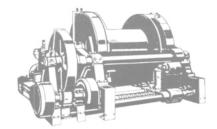
Heavy-duty Clyde with 36" diameter X 51" Face single drum. Flanges 68". CAPACITY: Up to 2800' of 2" wire rope. Normal line pull 40,000 lbs@ 50 FPM. Steam or air pressure required 125 to 250 PSI. Can be adapted to electric drive or increased steam or air pressure to a capacity of 82,000 lbs @ 20 FPM. Pawl holds 270,000 lb. pull from any layer. Equipped with level wind device. Approximate weight 30,000. DIMENSIONS: 12'6" wide—6'6" high. Write for details.
