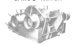
2-Speed — single drum — reverse throttle operation. LINE PULL: low gear 10,000 lbs — high gear 5,000. LINE SPEED: low gear 125 FPM based on 1st layer of 7/8" diam. rope — high gear 250 FPM based on 1st layer of 5/8" diam. rope. DRUM: 26" diam. — 20" long — 26" flange diam. Rope capacity of drum: 7/8" diam. rope in 6 layers 650"; 5-8" diam: rope in 8 layers 1200". Steam preassure at throttle 115 lbs. Operating weight 6450 lbs.
