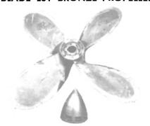
Starboard -7' diameter - pitch constant 4.699: Bore tapers from 6%'' to  $4^{5}\%_{4}''$ .  $14^{1}\%''$  taper equal to 1''/foot on diameter. U.S. Navy reconditioned. Average weight 1760 lbs.
