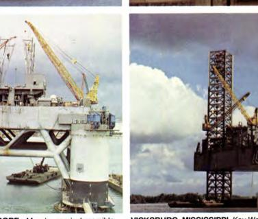
**REPUBLIC OF SINGAPORE** Margie, semisubmersible, twin hull, measures 202' long x 182' wide x 110' high; 9,000 tons. Designed to drill in 600' of water. Crew of 90. Scheduled to drill off the coast of Northern Australia.
