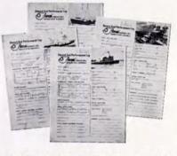
RECORD AND PERFORMANCE LOGS of all Demountable-fitted vessels go to 30 Johnson Reps around the world, and are regularly updated. Data includes vessel name, a photo, bearing locations and dimensions, drawing references—everything needed to expedite service at any repair yard. Copies go to ship's files. If you'd like to see some typical ones, drop us a note.
