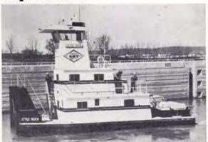
The twin-screw Little Rock, powered by a pair of GM Detroit Diesels, has push knees 12 feet high and a pilot eye level of 25 feet.
