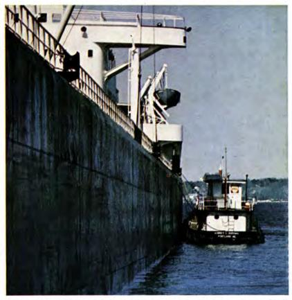
Golten Ship Repair tank boat, the Aubrey L. Hudgins, pumps Shell MELINA Oil into ship in mid-harbor at Portland, Maine. The Hudgins' pumps can deliver 4,800 gallons per hour from her 48,000-gallon-capacity tanks. Turnaround time for ships is speeded up by this fast, clean delivery system.
