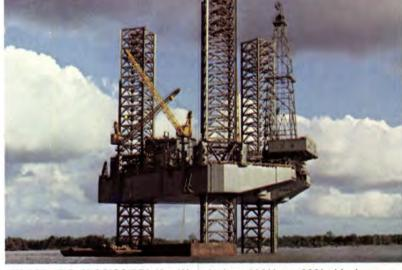
VICKSBURG, MISSISSIPPI Key West, jackup, 230' long, 200' wide, legs 467' high; 6,000 tons. Designed to drill in 300' of water. Crew of 97. Notice the three 45-ton marine cranes, usually on almost all rigs Marathon constructs. Scheduled to drill in waters off Belem, Brazil.
