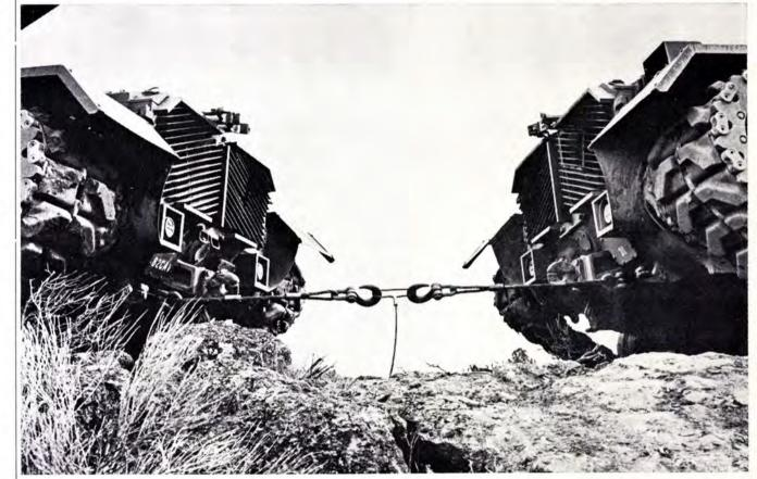
We put three different swaged sleeves through the toughest torture test we could devise: a side-pull test designed to tear wire rope slings apart at the sleeves. This is what happened: In a tug of war between two 52-ton tanks, the  $\frac{1}{2}$  " aluminum and carbon sleeves ripped apart, but the ESCO  $\frac{1}{2}$ " stainless duplex sleeve wouldn't give up.
