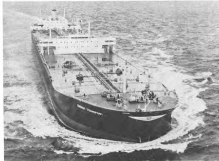
S.T. Energy Transport, shown above, is powered by a 30,000-hp General Electric MST-14 steam turbine gear propulsion equipment.
