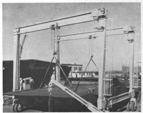
Traveling carriers move subassemblies from the motorized buildings to the pier for installation on the ship.
