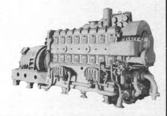
3-268A DIESELS - 150 H.P. @ 1200 RPM DRIVING 100 KW 3/60/440 GENERATORS COMPLETE - ALSO D.C. UNITS AVAILABLE
