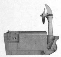
Model 02-D—powered by 6-cylinder G.M. 6-71 diesel—driven through Oliver gear—8708—forward ration 1:1.27—reverse 1:1—3 blade propeller—48" diameter—24" pitch—left hand—manual steering—electric starting. RECONDITIONED—READY TO GO!
