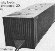
**Box Bulker** ISO container, with roof hatches and front end hatch for dumping.
