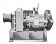
American Hoist and Derrick Company Winches with Westinghouse Motors, 50 HP, 230 Volts DC, complete with Contactor Panels, Master Switches, and Resistors. Type 66-single speed, single drum. Type 67-two speed, single drum.
