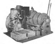
Small general purpose winches, mfg by Jaeger. Rated 2500 lbs @ 75 FPM. Driven by air-cooled Enfield single Cylinder diesel engine. Declutchable free spooling drum has center flange which can be removed if required. Excellent for small vessel use and general purpose service on all vessels. Has spare parts box. Weight about 1500 lbs.
