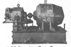
**AP3 Steering Gear Pumps** Northern Hydraulic (variable \$1750 stroke) and Hele-Shaw Hy-
