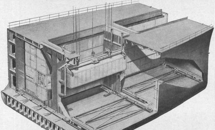
To take advantage of the efficiency of container shipping, Seatrain Lines, Inc., turned to the AAI Corporation with a basic concept to convert four C-4 cargo ships to container ships. AAI, with capabilities in electronic, mechanical and hydraulic materials handling systems, engineered and furnished much of the hardware for a hydraulic system which allows 24 containers to be loaded in each bay through a conventional hatch. This eliminated ex-
