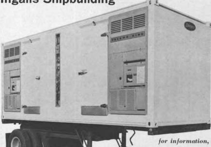
Pre-loading stores in Dorsey-designed refrigerated containers will help new automated ships cut days off port time.
