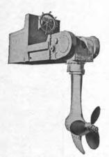
1 Model 0-7 unit in stock. Powered by twin GM 1 Model 0-7 unit in stock. Powered by twin GM 6-71 diesels with hydraulic clutch & electric steering. Propeller diam. 64" pitch 48". Tailfin raised & lowered mechanically. 7' from bottom of unit to propeller hub center. Weight about 20,000 lbs. Propeller speed 308 RPM. Unit can develop up to 500 HP. Formerly used on Cargill Grain Co. barge "Carpolis". Actual photo on request. Can be demonstrated running in shop.
