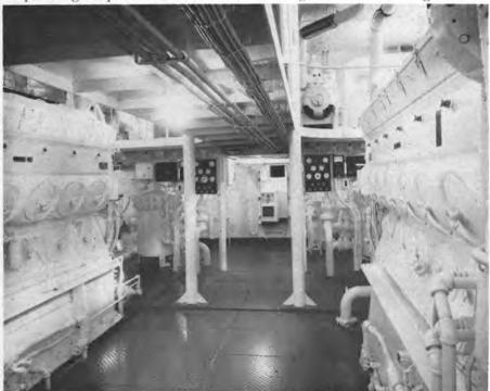
View down the centerline, looking forward, of the engine room showing the G-M diesels.
