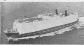
Aoi Maru can carry 737 Toyopet cars. The 380-foot 4-inch vessel has a beam of 53 feet 2 inches, molded draft of 16 feet 5 inches. It is equipped for stern loading.
