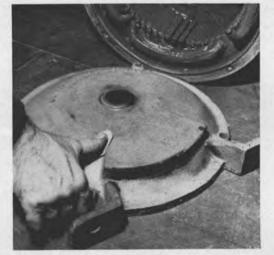
Electric Motor housing being repaired with EPOXY-BOND. Jobs like this are easy for EPOXYBOND—reduce maintenance costs.
