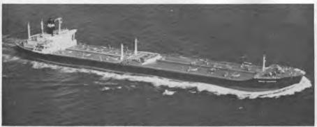
FIRST OF TWO 87,000-DWT TANKERS was recently delivered by Mitsui Shipbuilding & Engineering Co. Ltd., Tokyo, Japan, at its Tamano Works to Drummond Shipping Company of Monrovia, a member of the Niarchos group. The 810-foot vessel, World Kindness, is propelled by a 20,700-bhp, Type 984VT2BF-180, Mitsui B & W diesel engine which gave a trial speed of 17.2 knots. The second ship, World Knowledge, will be delivered this spring. Both vessels are classed by the American Bureau of Shipping.
