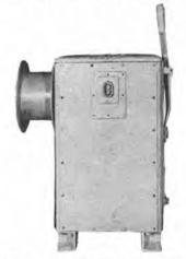
Designed for use with Bathythermograph—Submarine Signal Co.—type E/2/S—without cables—single speed 300 lb. pull @ 360 FPM—single drum 9" X 634"—with 1478" flanges—clutch controlled with pawl & ratchet. Designed for use with 1200 ft. of 1/8" stainless cable. Motor: 3 HP—440/3/60—1700 RPM—intermittent. 5 Availabe-Navy surplus-show little use.
