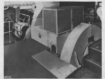
Figure 2—Synchronous generator fitted in line of shafting.
