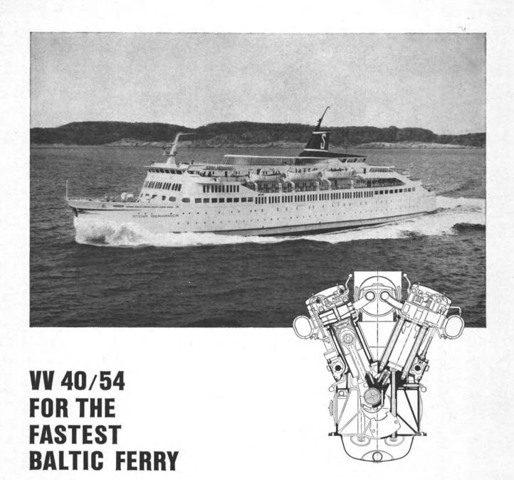
M. S., Stena Germanica" of Stena A. B., Goeteborg, is the fastest Baltic ferry to date. Two M.A. N. V8V 40/54 16-cylinder-engines, each with an output of 8640 BHP at 400 rpm, give the ship a speed of 23.5 knots. The ferry sails between Goeteborg and Kiel with a capacity of 1400 passengers and 200 vehicles. This
