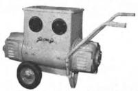
Motor: 10 HP—230 volts DC—2800 RPM. 200 amps max. continuous welding. Range regulation 15/200 amps. Dimensions: 38" X 30" X 20". Weight: 514 lbs. Shipping case—48" X 35" X 25". Complete with 100 ft. welding cable—ground clamp & electrode holder. Built to Lloyd's—Register BS 638—1954.
